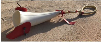
Figure 10: Pufferfish prototype (version 2 with one handle and flexible plastic parts attached resembling fins and a tail).
